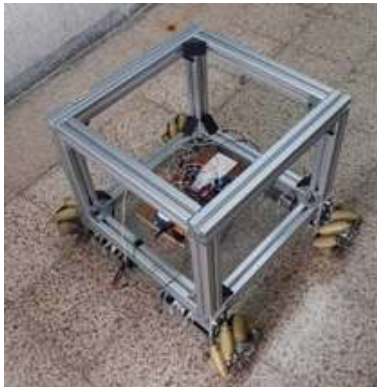
Fig. 5. Robotic base photograph and it's components.
