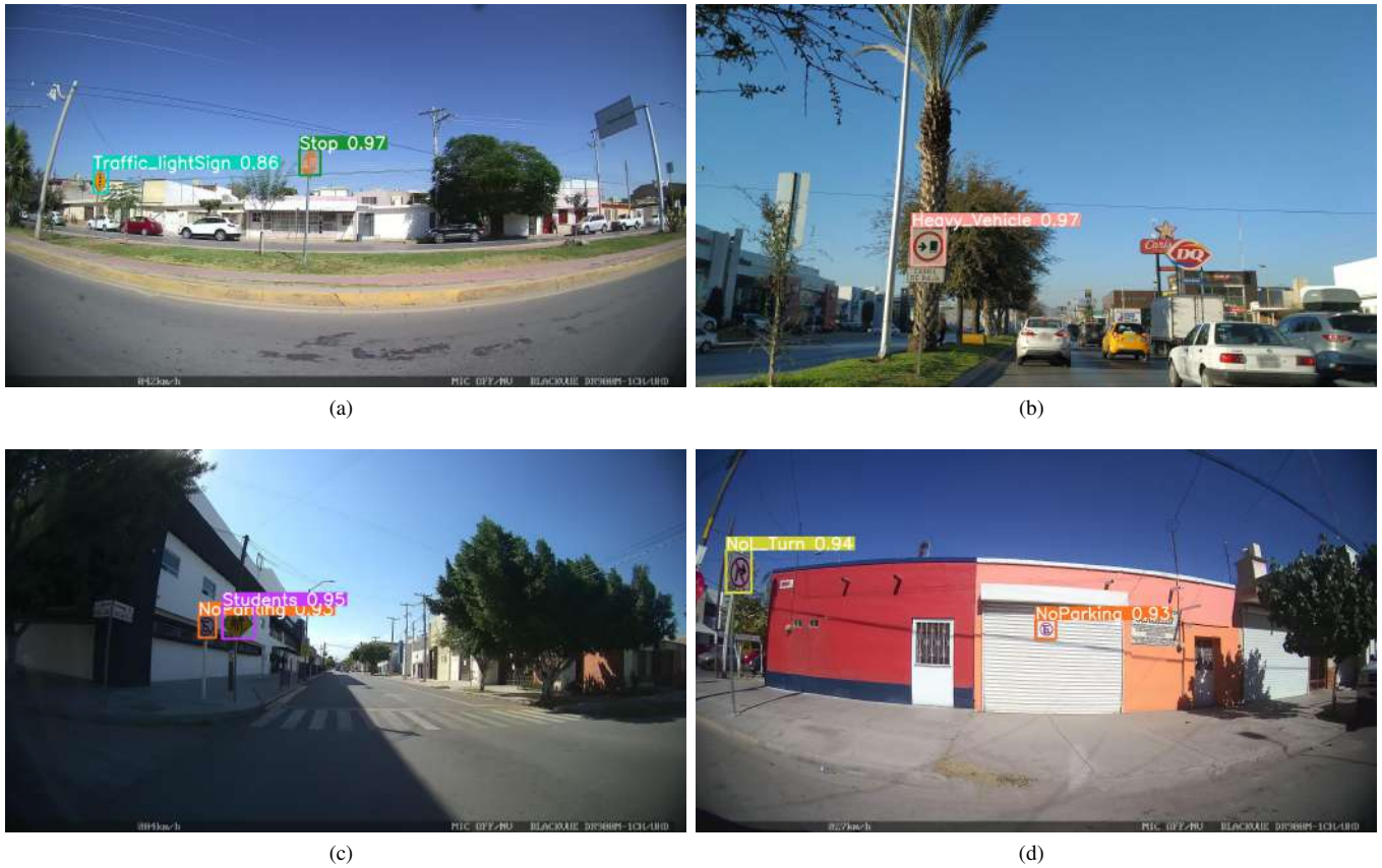
Fig. 3. TSD detections: (a) “Traffic_lightSign” 89% and “Stop” 97% (b) “Heavy_Vehicle” 97% (c) “NoParking” 93% and “Student” 95% (d) “NoL_Turn” 94% and “NoParking” 93%
