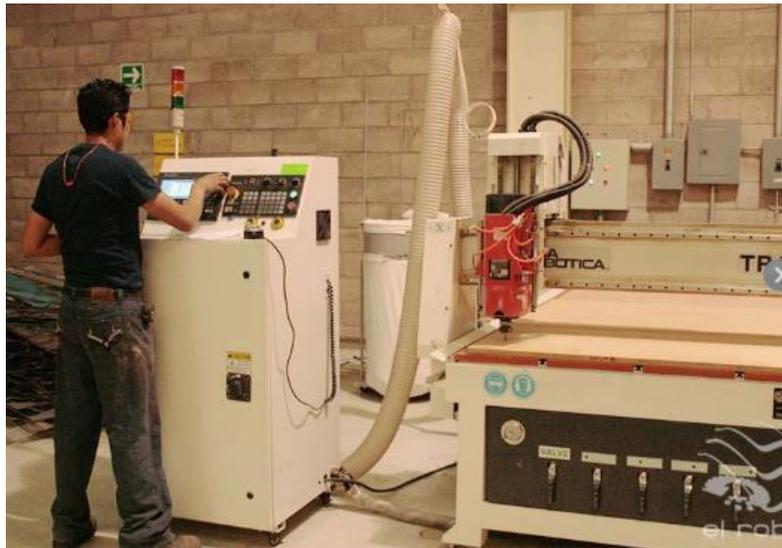
*Figura 1.7 Router CNC*
