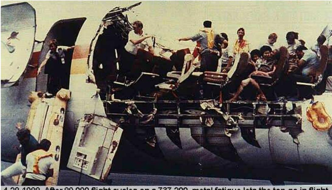
*Figura 1.9. After 89,090 flight cycles on a 737-200, metal fatigue lets the top go in flight (28-abril-1988)*
