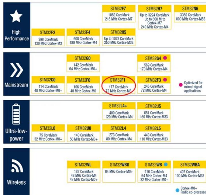
Figura 8.1: Procesadores Arm Cortex-M de STMicroelectronics.
