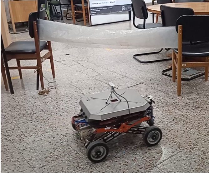
Fig. 14: Testing scenario for obstacle avoidance with the RGB-D camera.
